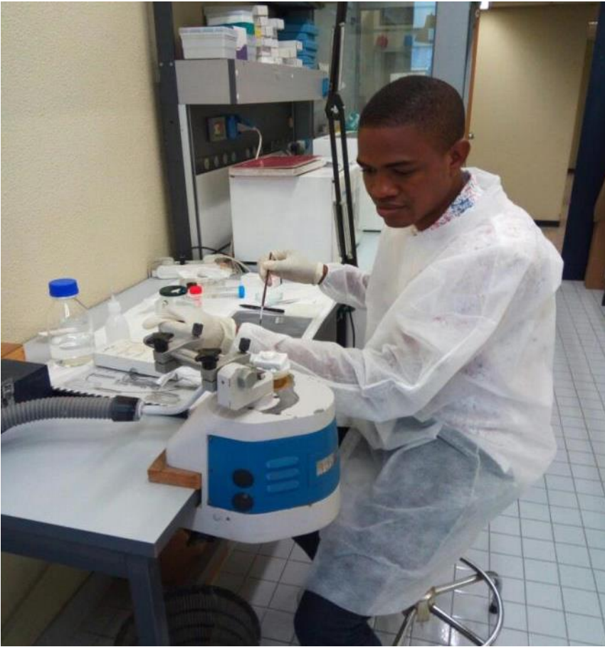
My picture while sectioning with the freezing microtome in the lab at the University of Verona.
